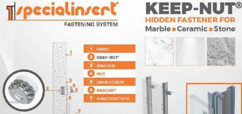
Specialinsert® Keep-Nut® is ideal for the production of wall coverings, ventilated facades and countertops. It is made of stainless steel and it creates a threaded seat in all stony materials, simply applied by pressure into a standard cylindrical hole. It is ETA certified and ASTM tested.
