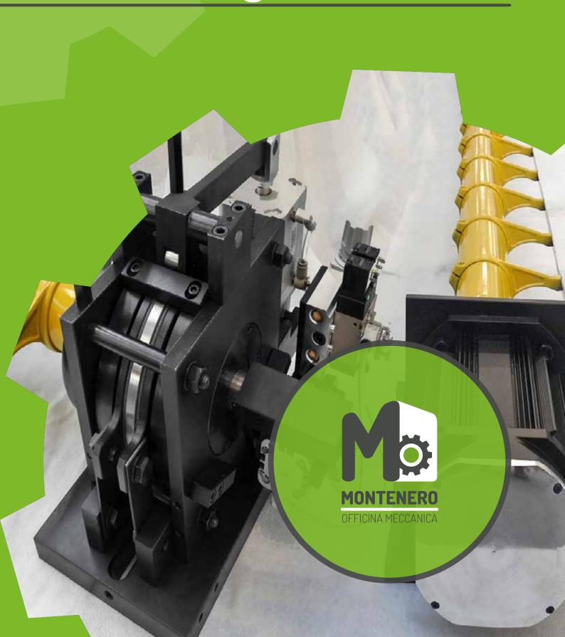
A new generation of fly comb systems: Electronic Generation Over 3500, electronically controlled doffing concept. This sysem is able to pass 2950rpm with a stroke up to mm55. Available with a working width up to 3,5mt without central support.
