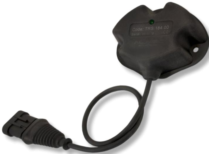
The TRS.184 is an inclinometer sensor based on a double CPU, a double 3D-MEMS accelerometer and a double gyroscope, in a fully redundant circuit scheme.
