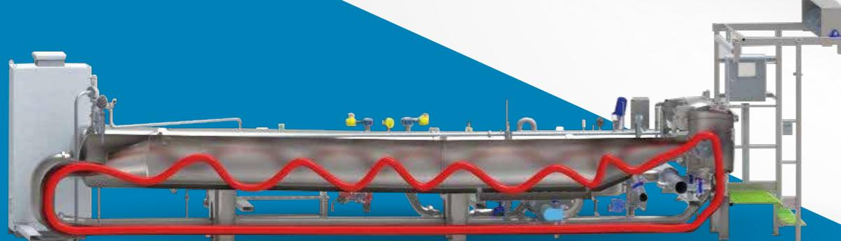
Four variants tube diameters for smooth move of the fabric
