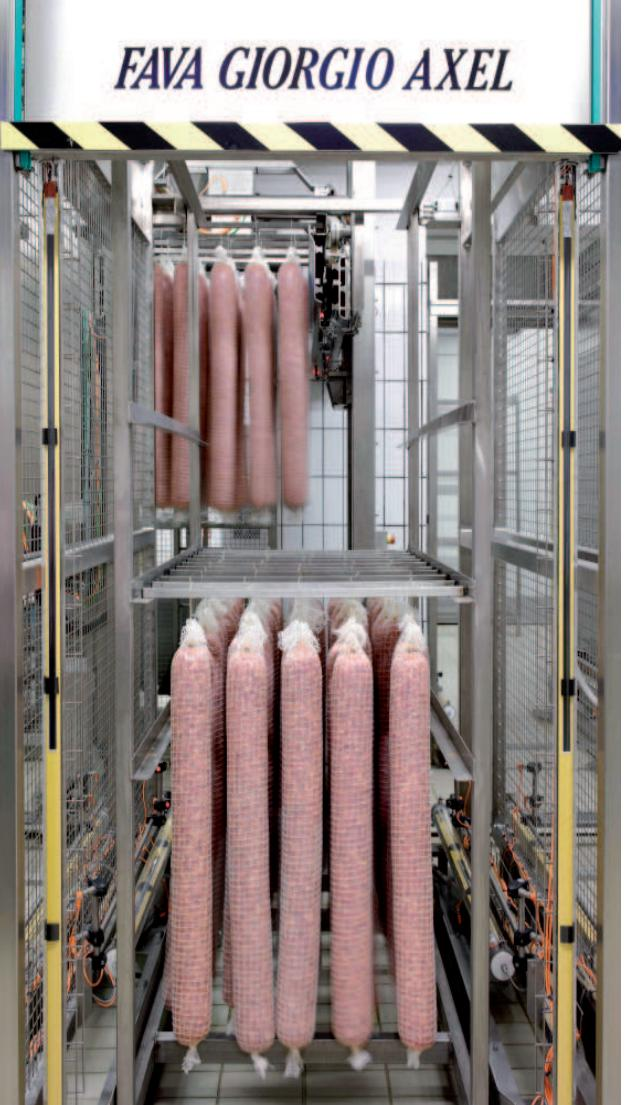
TFRC can be used even for cured ham both lying during salting phases and hung in the following production phases. TFRC can connect the normal front-back working modality with the possibility to make rotations of the product around the vertical axis, always with oscillations control and in the smallest possible space.
