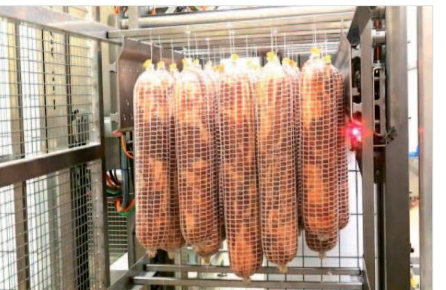
TFRC can load and unload very high trees, trolleys, racks and frames moved by LGV or by overhead rail system, independently from the loading height. During the unloading phase it's moreover possible to unload one by one bars to feed packaging and peeling lines or to automatically extract bellies from the hanhing combs to feed pressing lines.
