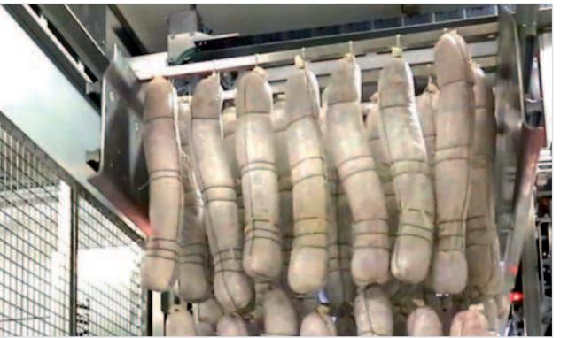
Our plants can be fed by our automatic or semi-automatic loading devices. The salamis loading can be done manually, anyway with no effort for the operators, or automatically with machines that can be connected to the customers' filling and clipping lines.
