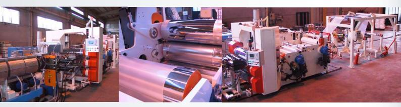
Our COMPACT exp series is another specially designed extrusion lines family for the production of EPP & EPS Sheets, by a successful mixing-recipe of standard PP/PS with Chemical Blowing Agents (CBA). This family of extrusion lines is expressly studied to grant a perfect and homogeneous foaming of the PP & PS along the complete width of the sheet.
