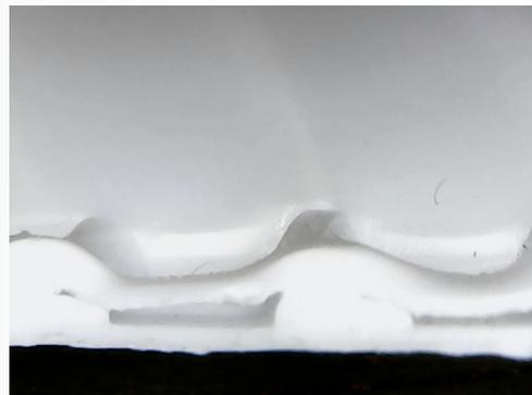
FIG.2 200X magnification of a seal performed with traditional hot-die cutting machine.
