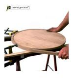
Bendywood® should **always** be bent **around a mould**. To this end you can use clamps, presses, tension belts, etc. and then you should wait until the bent form has stabilized, best by drying it to 8% final moisture content. Pictures of moulds can be seen on our website under the rubric "<u>Bending moulds for Bendywood®</u>".
