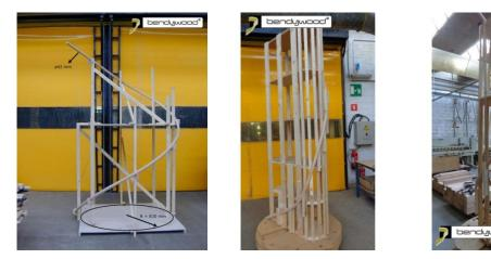
In case it is not possible to use the staircase itself as bending mould, you can build a mould as shown in the above video and pictures. Keep the radius about 10% to 20% tighter than the requested final radius, as the bent handrail will always "open up" when taken from the mould.
