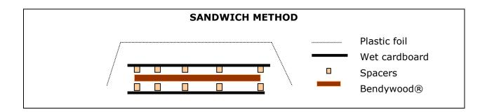
Using this technique (referred to as "Sandwich Method") the Bendywood  ${\ensuremath{\mathbb R}}$  absorbs humidity form the air without getting wet.
