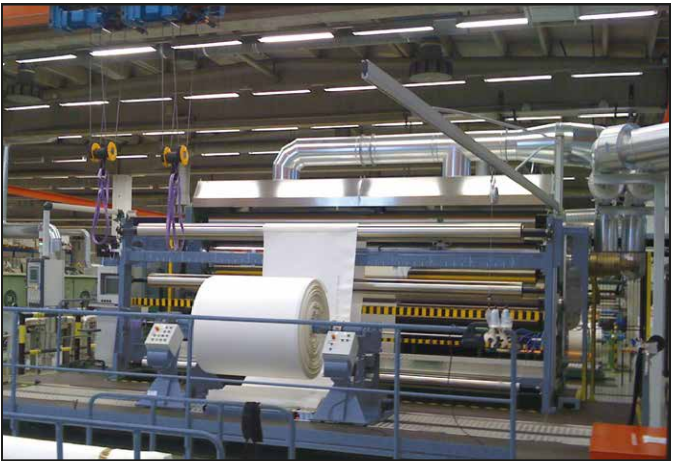
Nipco™ HT 5.200 mm roller width
