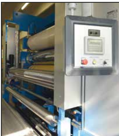
Movable satellite operation panel
