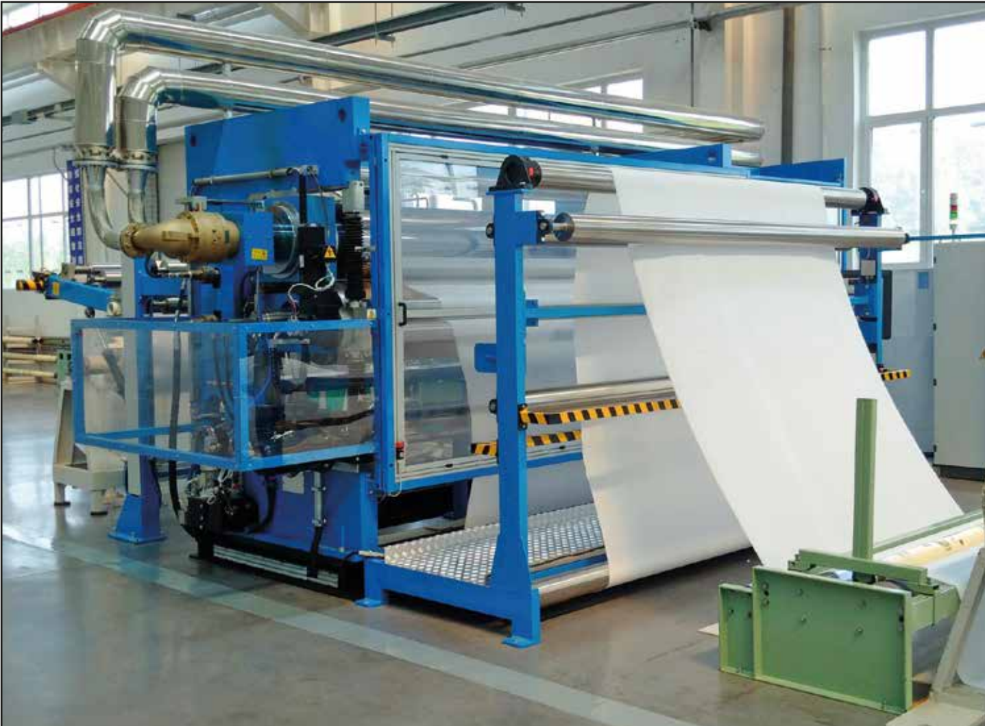
Nipco™ HT I 2 bowed version roller width 3.600 mm.
