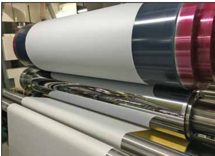
Nipco™ bowl with paper sleeve and Nipco™ zone controlled pressure setting bowl with TopTec3 sleeve Drive side
