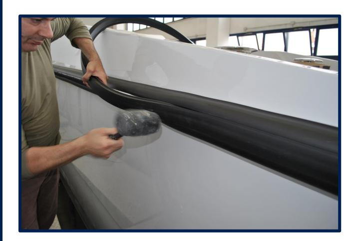
The product can be assembled very easily: after fixing the base as previously mentioned, the "top" is pressure fitted with a rubber hammer.
