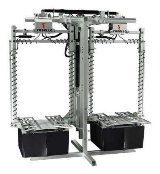
The implement is designed to fit on the front of the tractor, featuring a straddle frame so that you can treat two rows at a time. It features six hydraulic cylinders for adjusting the lift, side shift, head opening, and angle. It also has a suspension system for smoother running over uneven terrain. The unit comes with suckering heads fitted as standard, while the mounts for rubber cones for under-vine weed control are optional extras.
