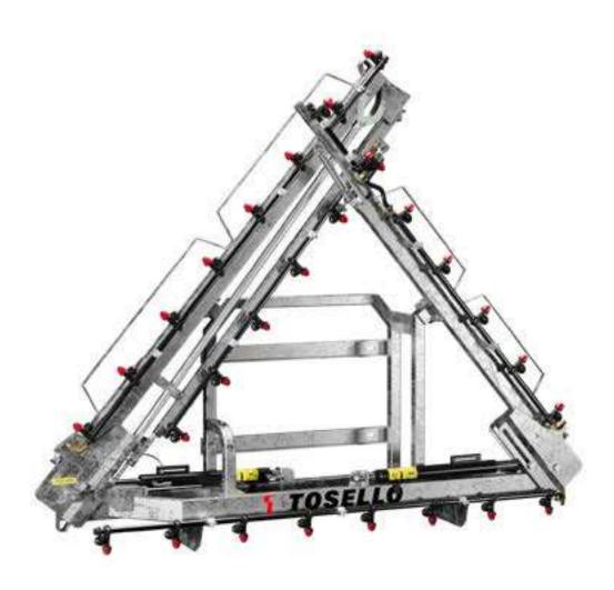
Weed spray boom to be attached to existing weed control units, or for use in conjunction with our linkage sprayers. Its distinguishing features are its perfect size for greenhouse use — measuring 7.5 m across in asymmetrical mode — and its hot-dip galvanized treatment, which protects the frame from corrosion from the chemicals used.
