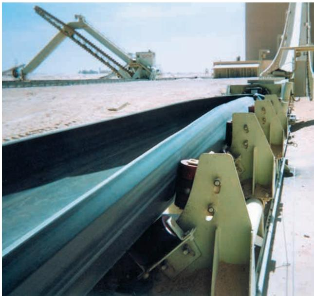
Pipex and Piflex are conveyor belts designed for tubular conveyor systems equipped with a textile or a steel cord carcass, respectively.
