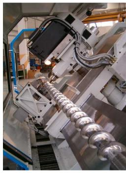
The bed is in electrowelded steel structure stress relieved with grinding surfaces to hold high precision guideways for rollers sliders.
