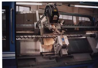
The models SAPORITI PLUS 400 are equipped with CNC, motors and drivers Siemens. The milling head motor power is 22 Kw. The spindle nose is ISO 50. Max spindle speed 5000 rpm.
