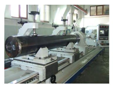
There are six controlled axis, four linear, Z1 longitudinal length of the machine, Z2 longitudinal of steady rest (lapping head optional), X1 transversal first carriage, X2 transversal second carriage and one rotary, S1 rotation drilling tool.
