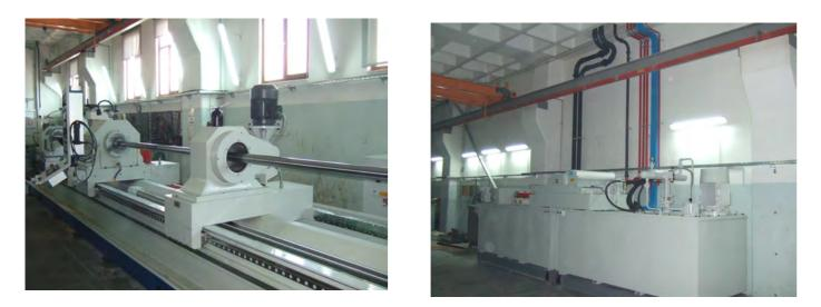
The Main Settling tanks can hold up to approx. 6000 Litres of Neat Oil and is accessible through the removable top plates. Each tank is divided into smaller sections of baffles and both are united via a transfer tube. There is a 37 KW Motor drives a Gear-pump, for the hydraulic circuit
