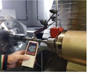
The ball valve grinding machines PV500 have the positioning Y vertical axis of the grinding head. This axis allow to make micro movements CNC controlled, with a maximum stroke of ±1 mm for the perfect alignment between the grinding wheel and the ball centre. This extremely important feature allow to obtain the best accuracy during the working process. In fact roundness accuracy better than 0.01 mm and roughness better than Ra 0.2 µ can be easily reach.
