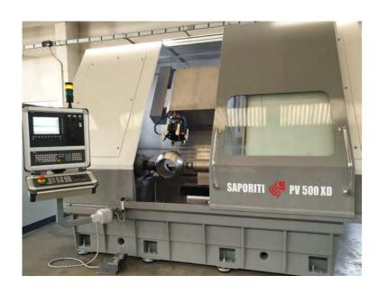
The SAPORITI PV500 series is supplied with suitable anti-vibration supports to be easily placed on standard good industrial floors without any foundations works. The filters can be placed on floors in position defined with the Customer.
