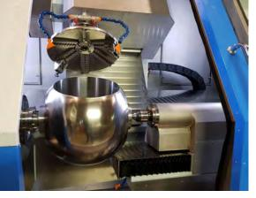
The tool holders wheels have hydraulic nose HSK A 100 or 125 (optional) for rapid tool changing. They are supplied with a suitable arm to hold them in an inclined position for the easy interchanging on the machine grinding spindle where there is an hydraulic tool clamping. Grinding wheel changing is fast and easy.
