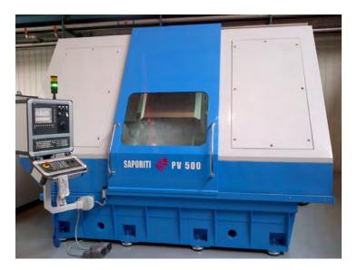
These machines are on high precision roller sliders assuring the longest machine life time and the highest accuracy in order to obtain the workpiece best roundness and roughness.
