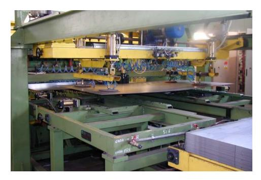
System for **profiling and piercing the multiple plate** in various sizes, obtained with die changing only. A particular system enables bending and piercing two plates at a time, up to a maximum width of 8 mm.
