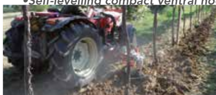
• Self-levelling compact ventral hoe (Lotti patent since 1980)
