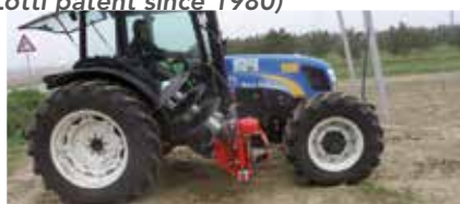
• Self-levelling compact ventral hoe (Lotti patent since 1980)
