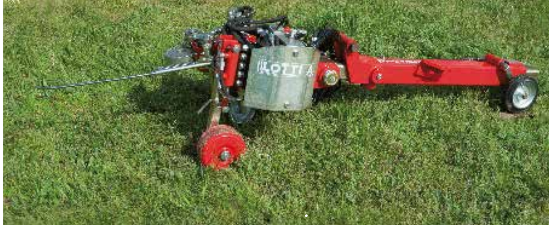
• Self-levelling compact ventral hoe (Lotti patent since 1980)
