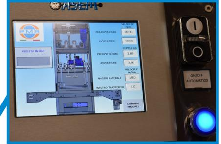
**Touch-screen panel** for setting and storing all parameters and adjustments.
