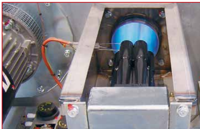
Bruciatore Ecomix - patented Multiventuri technology Ecomix Burner - patented Multiventuri technology
