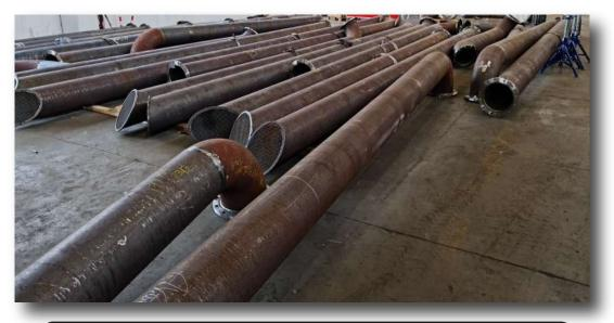
Carbon steel prefabricated piping
