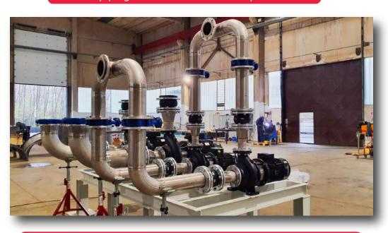
Skids complete with electrical panels and PLC
