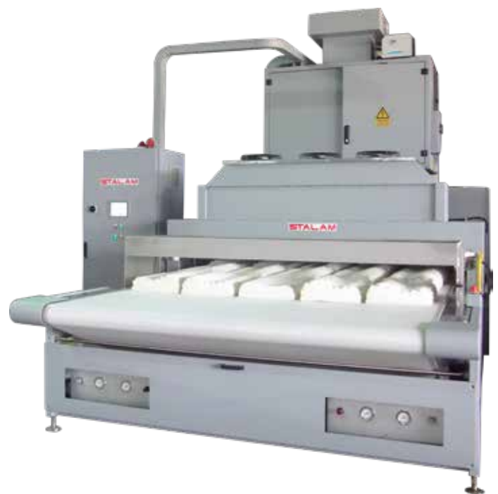
"RF/A 105 kW" model dryer with 2.2 m wide conveyor belt for natural latex mattress cores and pillows.
