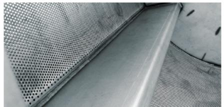
is completely made of 5 mm thick AISI stainless steel, properly perforated to guarantee a perfect cycle of the bath inside the drum
