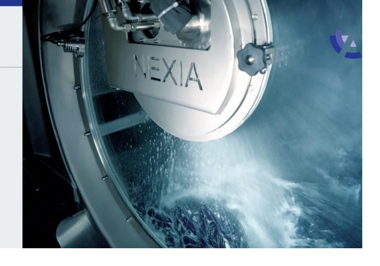
The water is collected and re-injected through these injectors with a pressure suitable for the treatment of the denim
