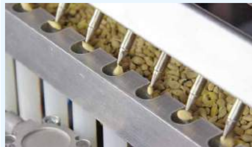
Sowing nozzles can also sow large seeds , such as those of citrus fruits .
