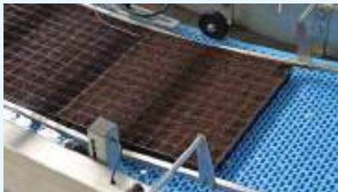
Corrosion-resistant polypropylene (PP) conveyor belt.
