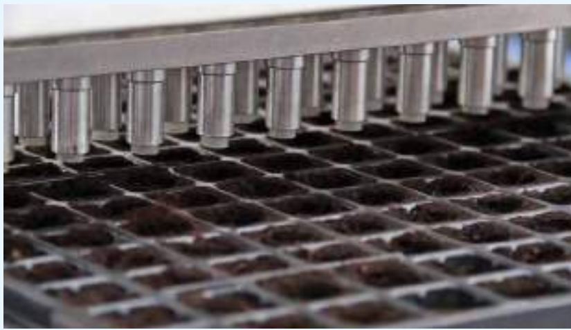
KAPPA65C seeding line with double row seeding nozzles.
