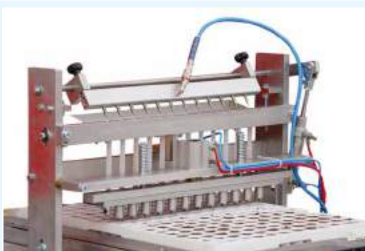
Seeding bar kit assembled on the seeder.
