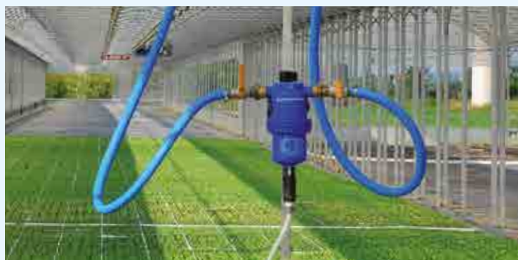
Proportional dosing unit directly assembled on the irrigation boom.
