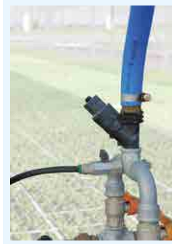
Water distribution group with ball valves for side nozzles and pressure regulator.
