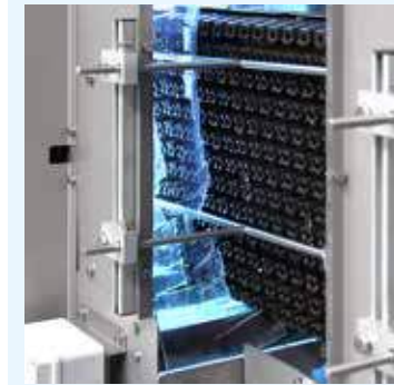
Trays treatment tunnel with UV lamp system .
