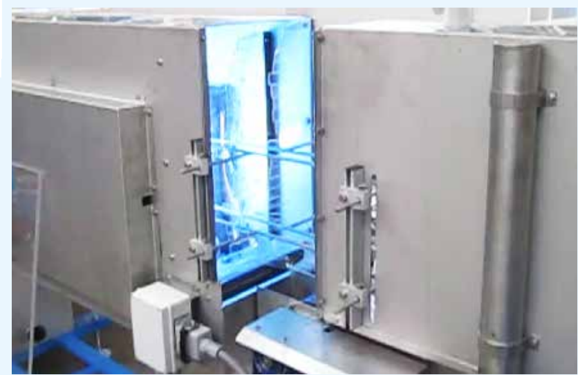
Trays treatment tunnel with UV lamp system .
