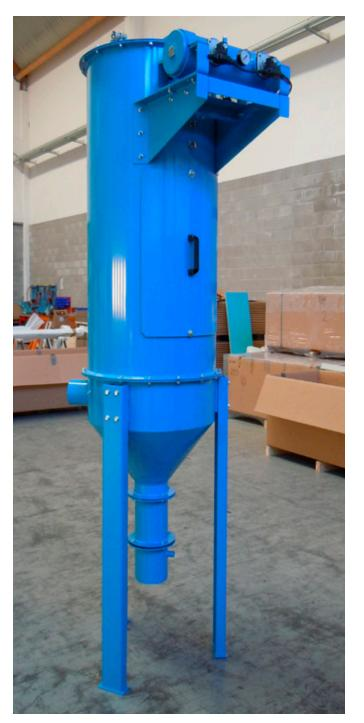
Cylindric HSS (High efficience), filter-unit. Two or more levels of filtration
