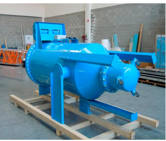
Filter-unit with absolute filters, 1 or more filtering levels
