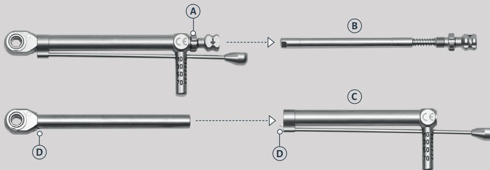
The dynamometric ratchet, after each use, must be disassembled for cleaning. This maintenance operation does not require any tools. Completely unscrew the screw **(A)**, remove the whole pawl **(B)** and then the flexible dynamometric bar **(C)**. Once disassembled, clean according to the instructions for use
