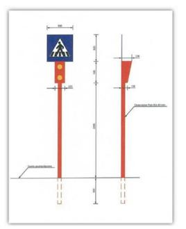
"P.S./Intelligent Crossings' is a signalling system for pedestrian crossings not already covered by traffic lights
