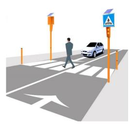
The central body of the system will be positioned close to the pedestrian crossing, by means of two signal poles, one on each side of the crossing, equipped with photocells which, when the pedestrian approaches, will trigger the entire control and management system of the flashing lights.
