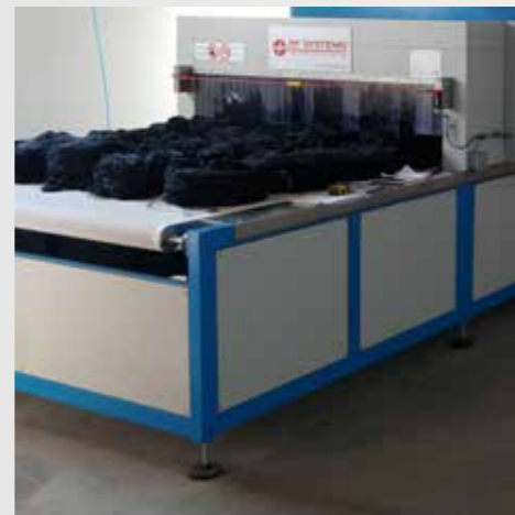
> RF drying of tops 3 Ton/day throughput
