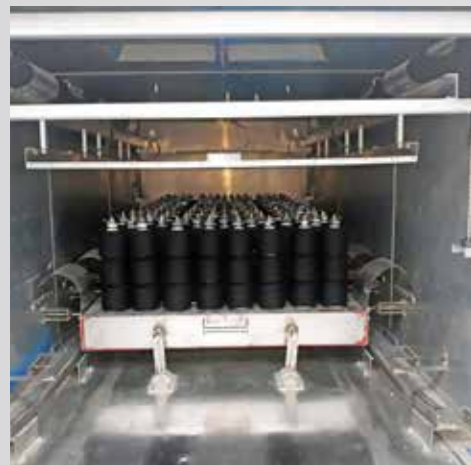
> RF drying of bobbins 3 Ton/day throughput
