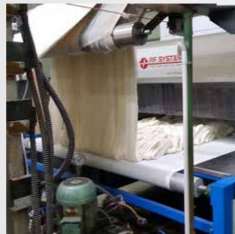
> RF drying of slivers 2 Ton/day throughput
