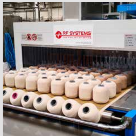
> RF drying of yarn packages 7 Ton/day throughput
