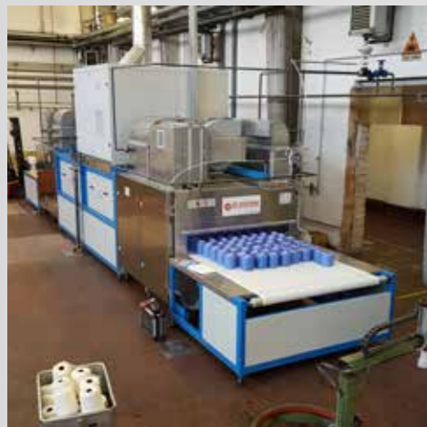
> RF drying of yarn packages 4 Ton/h throughput
