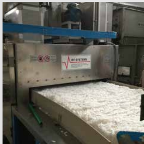
> RF drying of loose stock 600 Kg/h throughput
