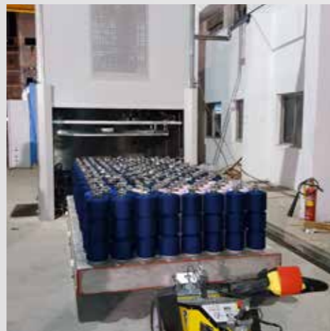
> RF drying of bobbins 6 Ton/day throughput
