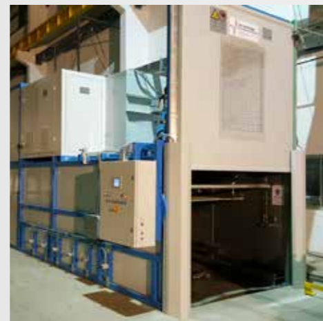
> RF drying of bobbins 5 Ton/day throughput
