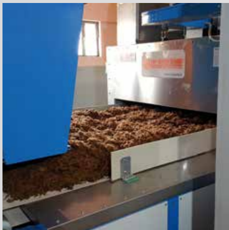
> RF drying of loose stock 800 Kg/h throughput
