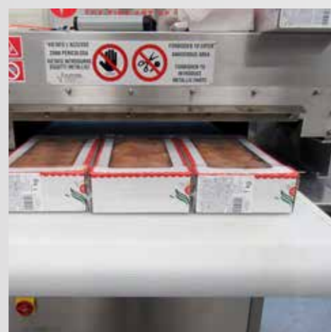
➤ Pasteurization of packaged croissants 300 Kg/h throughput
