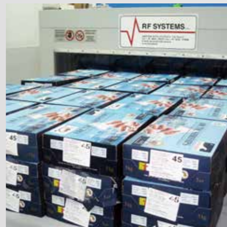
> Defrosting of packaged shrimps 1500 Kg/h throughput
