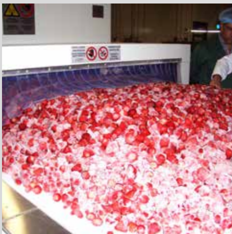
> Defrosting of IQF strawberries 1000 Kg/h throughput
