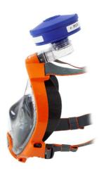
2. In combination with the Aria Protection Adaptor (APA), the RD40 40-22 mm adaptor (conical connector 22mm - ISO 5356-1) and an HEPA filter (standard thread connector EN148-1, RD 40-1/7"). This kind of filter protects against airborne and liquid-borne microbial pathogens. For more info on filter, see the HEPA filter technical sheet.
