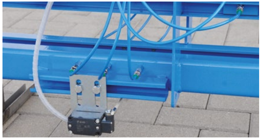
lubrication system for power & free conveyor
