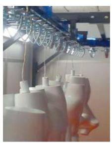
The monorail conveyor (type X37) is at the service of a mannequins painting line and leads the pieces to be treated along all phases of the painting process up to the unloading area.
