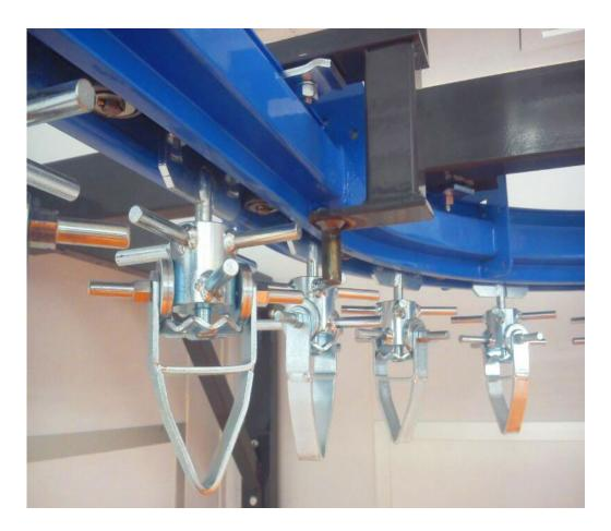
Rotating hooks with multiple spring-latches at 45° with 200 mm spacing.
