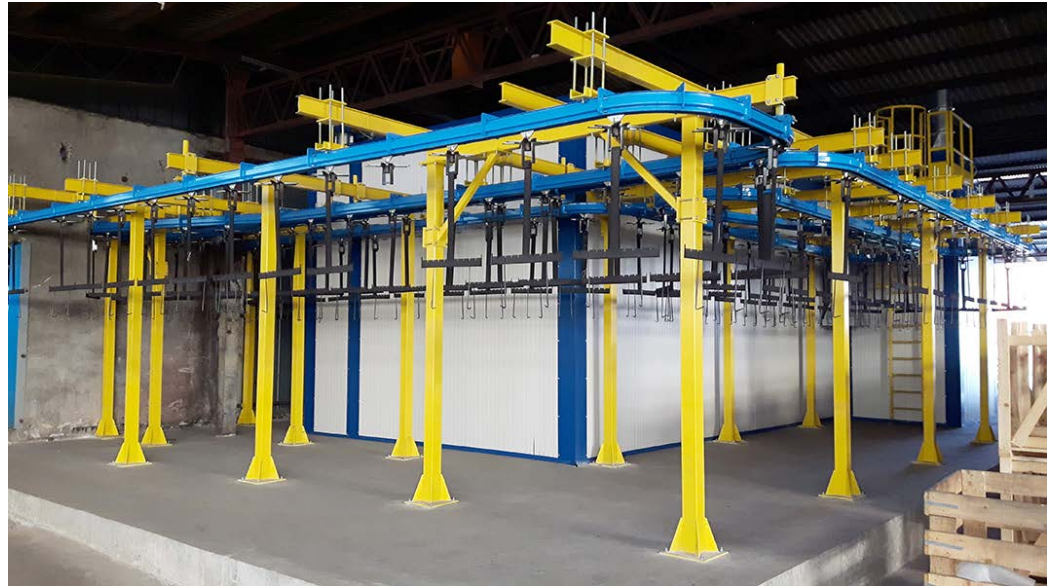
Overhead conveyor for painting line of cast iron pieces.
