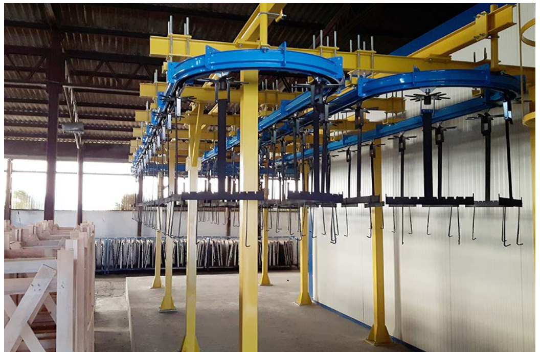
Rotating hooks with multiple 90° step, 600 mm itches.
