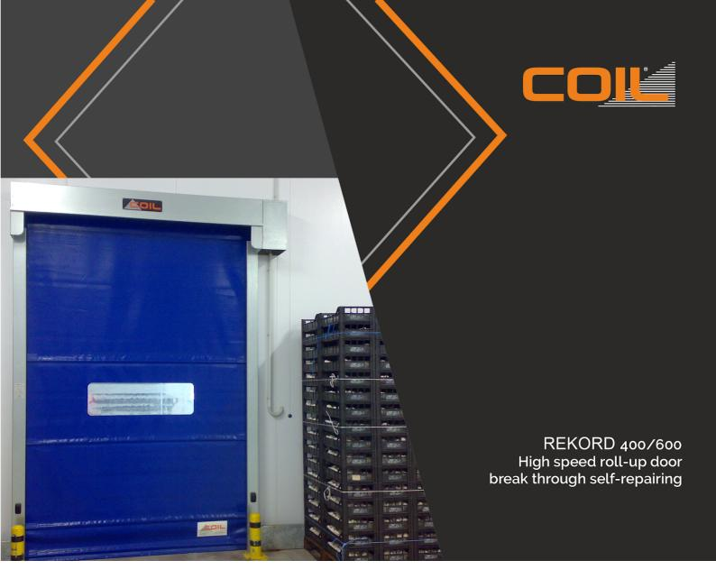
Equipped with a breakthrough system with automatic reset, in the event of accidental impact the mantle comes out of the sliding guides without being damaged and continues to operate by rewinding the mantle on the upper shaft. At the next closing cycle, and without any action by the operator, the mantle is guided back into the uprights. Ideal for installations as an indoor partition for commercial and food and chemical pharmaceutical production environments.
