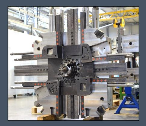
Tool detail - EV motor housing
