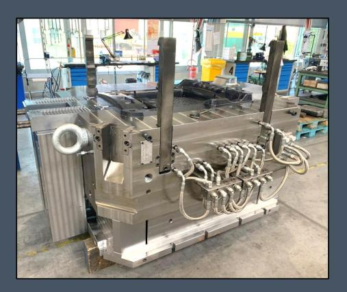
Tool - Inverter/Battery housing
