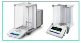
Analytical Electronic Balance with underplane support weight to position the support sample in the measurement area of the MVS2pro. The balance suggested is 5 decimal places in grams like: MS, XSR, XPR series (d= 0,01 mg). The Balance is directly controlled by MVS2pro via USB
