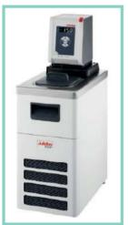
System of thermostatation for the beker (beker thermostatable). It allows the maintenance of the liquid measurement at the temperature described in the method. The system has a suction pump to recirculate the thermostated liquid in an external circuit and it is directly controlled by MVS2pro via USB.
