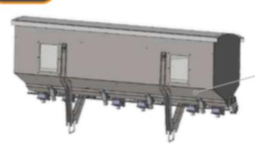
Fertilizer spreader for the distribution of granular products, with volumetric metering unit with mechanical drive and stainlesssteel tank. The distribution amount may be adjusted by the metering unit partition or by modifying, electronically or hydraulically the metering unit rounds per minute
