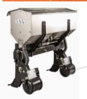
FERTIVITIS is a fertilizer spreader that allows to insert the product into the soil between the rows of vineyards or orchards. FERTIVITIS has a rigid toolbar and a stainless-steel tank. The blade coulters are equipped with depth gauge toothed rollers. It is available in 1 or 2 rows version. The working row spacing available on the 2 rows models, is either 1.4 or 2.00 m.
