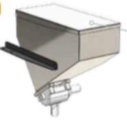
The MICROLINE is a volumetric metering unit suitable for the localized distribution of micro-granular products. A metering roller with flexible cells allows the distribution, while the adjustment is made through a partition controlled by a rotating ring nut. MICROLINE is easily adaptable to any farming machine and can eventually, be supplied with electric drive.
