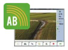
**A - B CURVE** - the program can create a sequence of curve pallel lines. They can be parallel to the first AB line or to the last one. The software can also create round lines suitable for PIVOT irrigation
