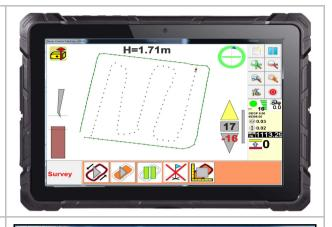
At the end of the survey, you can see immediately the land elevation (cut and fill area).
