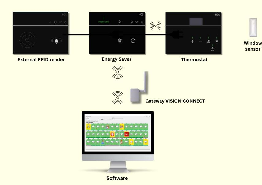
The wall reader is installed on the wall outside the room, and it is connected via RS485 to the internal reader. It opens the door when the RFID card enabled during check-in approaches. LEDs show the presence of the customer in the room, the activation of "Do Not Disturb" and the request for cleaning. It is also equipped with a bell.
