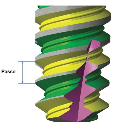
Means that the system at each turn screws twice the value of the *Passo della Spora*.
