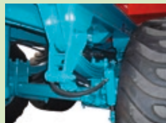
Telaio in HE con sospensioni paraboliche. HE beam steel chassis with parabolic suspensions.
