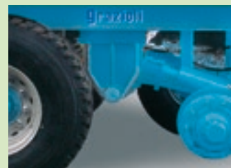
Assali tandem, balestre cantilever frenatura idraulica Tandem axles, cantilever leaf-spring suspensions, hydraulic brake system.
