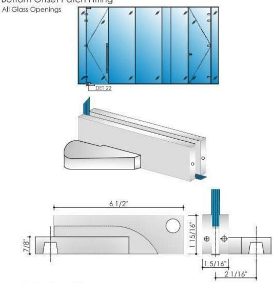
Hardware Characteristics Maximum Door Width; 42" Maximum Door Height; 102" Maximum Door Weight; 194 lbs
