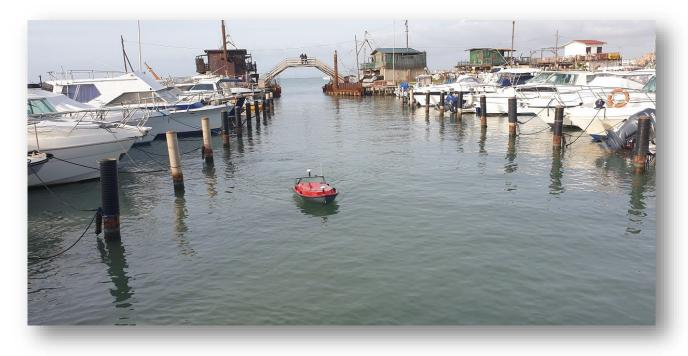
The CK-14 is an ASV, CE Marked, used for various hydrographic applications in inland (rivers, lakes, dams, artificial basin etc.) and coastal waters (harbours, coastal areas, etc.). The vessel is equipped with a large moon pool where many scientific instruments can be placed. Ready to use, customizable with a wide range of hydrogaphic and oceanographics sensors.
