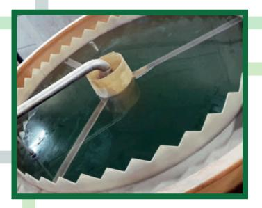
Through the chrome recovery system developed by **Deltacque**, it is possible to reuse the discharged baths in the tanning phases, separating and purifying with simple operations and with a low cost the chrome liquor, that can be reintegrated also in the process cycle, characterized by excellent quality standards.
