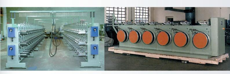
The SPINNINGPLANTseries is equipped with the SIEMENS CPU series 1500 and the whole production process is supervised through a touch operator panel managed by the software developed by AGRIPAK technicians on a SIEMENS TIA PORTAL platform.
