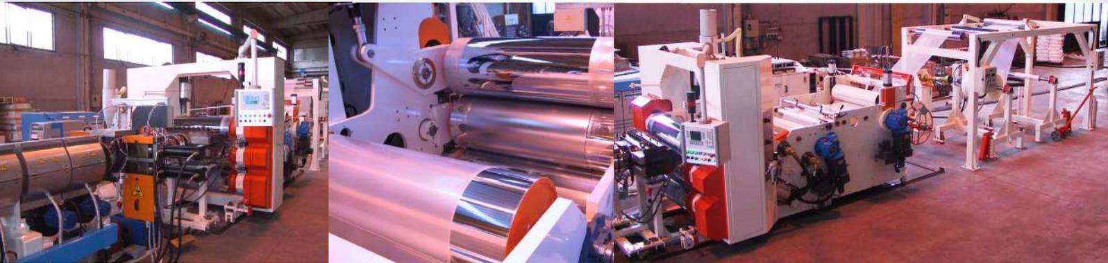
Our COMPACT exp series is another specially designed extrusion lines family for the production of EPP & EPS Sheets, by a successful mixing-recipe of standard PP/PS with Chemical Blowing Agents (CBA). This family of extrusion lines is expressly studied to grant a perfect and homogeneous foaming of the PP & PS along the complete width of the sheet.
